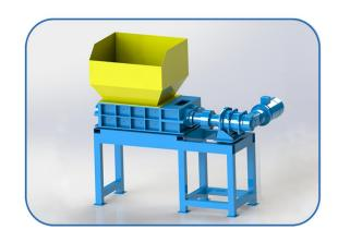
D series double shaft shredde has two rotors built into the machine that rotate at low speeds, high torque and low noise. With the function of PLC microcomputer control system, it is possible to control automatically start, stop. Automatic reverse sensors to protect the machine against over loading and jamming.
