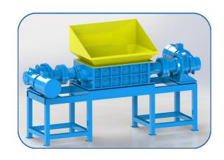
With the function of PLC microcomputer control system, it is possible to control automatically start, stop. Automatic reverse sensors to protect the machine against over loading and jamming.
